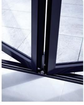
A unique, pivoting axle in the rollers allows the wheels to follow any undulations in the stainless-steel tracks underneath. Combined with sealed bearings in the stainless-steel wheels and lateral rollers, the doors will glide effortlessly and smoothly for years to come.
